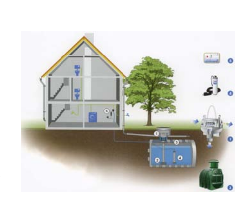
Typical domestic system schematic; commercial systems follow the same principles
